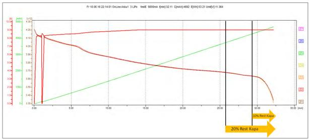
**Figure 1:** Typical voltage development of a lipo battery used in a racing boat at low load approx. 2C.
